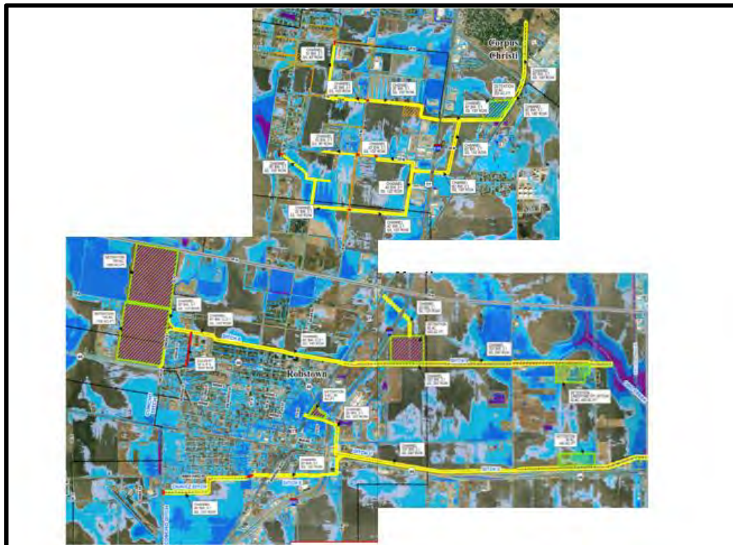
Figure 13. Proposed Conditions Model Inundation Boundary (North Robstown, West Robstown, & East Robstown Drainage Improvements)
